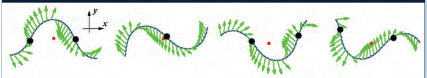
(Top) This side profile of a slithering snake shows that the creature lifts parts of its body from the surface while moving. (Bottom) A visualization of the calculated propulsive forces on a model snake with arrows indicating the direction and magnitude of the propulsive force applied by the snake to the surface.
