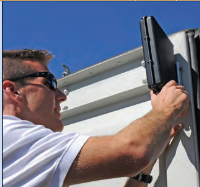
Top: GTRI's Container Security Device is shown being installed on a test cargo container. The device detects unauthorized door openings.
