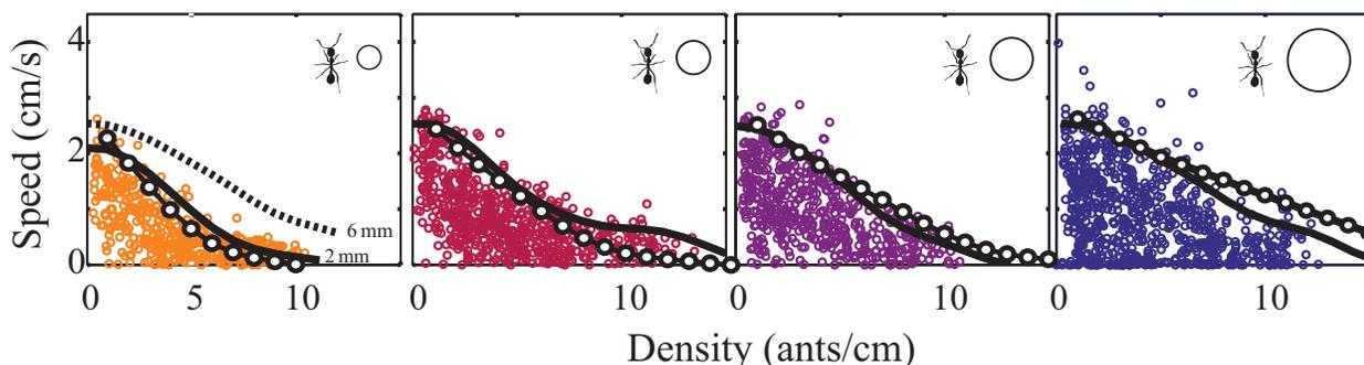
**Fig. 1** Fundamental diagram of bi-directional traffic flow in tunnels. Tunnel diameter increases from left to right. Solid lines are estimates of the bounding curves for the speed-density relationship. Dashed line in left panel is for comparison between 2 mm and 6 mm tunnels. Black and white circles are results from simulation for simulated tunnel diameters of  $D_{eff} = 2, 3, 4, 6$  from left to right.
