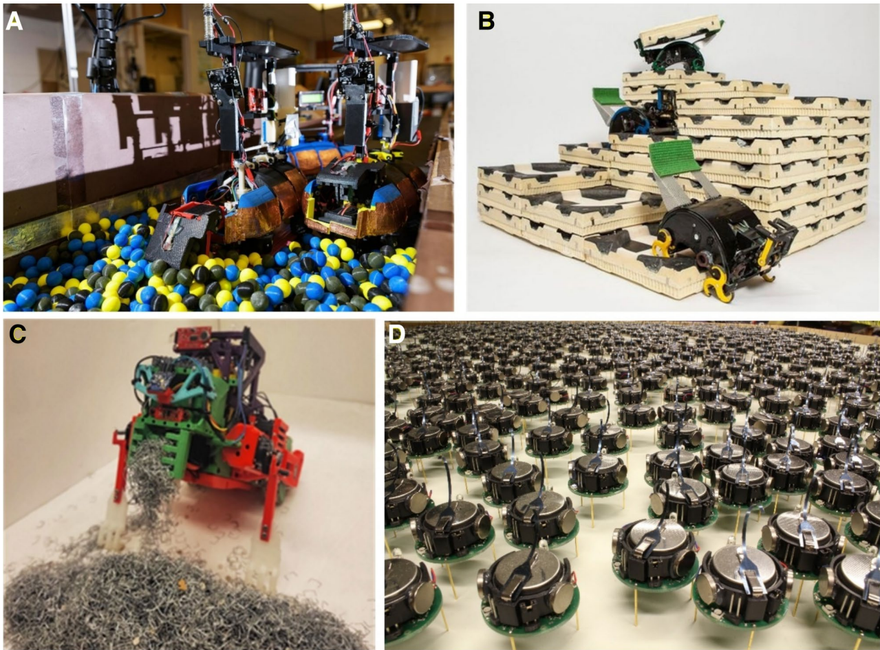
Fig. 6 Robotic systems used to model construction behaviors of insect societies. A Robophysical models struggle to excavate model soil in confined conditions. Photocredit: Jeffrey Aguilar, Daria Monaenkova, Vadim Linevich, Will Savoie. B Demonstrations of autonomous robotic construction with building blocks. Photocredit:
