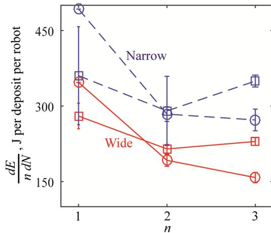
**Fig. 7** Experimental (square markers) and simulated (circular markers) energy consumption per deposit per robot rates plotted versus the number of robots in the system for a wide (3 BW, solid line) and narrow (2 BW, dashed line) tunnels. Error bars indicate standard deviations
