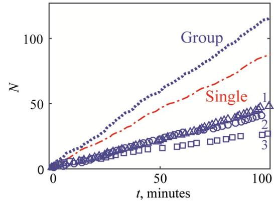
**Fig. 5** Number of deposits performed in a wide tunnel experiment (3 BW) by a robot excavating alone (dash-dot line), by individual robots excavating in a group of three (empty circles, triangles, squares), and the net excavation effort of these three robots (dotted line) as a function of time
