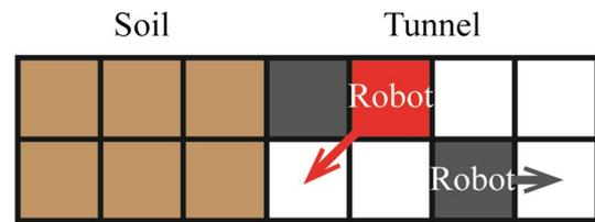
**Fig. 3** Schematic of the cellular automata model for a 2 BW tunnel. The cells in the model are in one of the four states: soil (brown), tunnel (white), ascending ant (gray), descending ant (red). In experiment, width of the narrow tunnel is slightly larger than 2 BW and is equal to 41 cm (color figure online)
