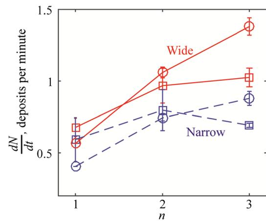
**Fig. 6** Experimental (square markers) and simulated (circular markers) excavation rates ( $dN/dt$ ) of systems with different number of robots ( $n$ ) in both narrow (2 BW, dashed line) and wide (3 BW, solid line) tunnels. Error bars indicate standard deviations
