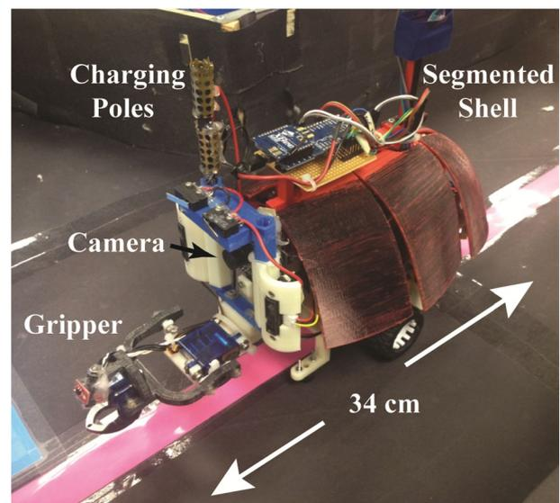
**Fig. 2** Robotic excavator with important components labeled
