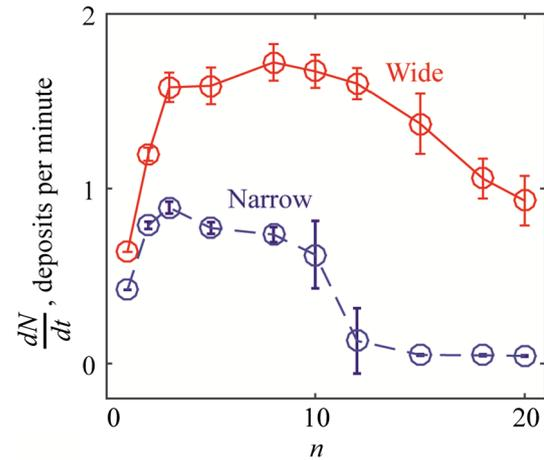
**Fig. 8** The dependence of excavation rate ( $dN/dt$ ) on the number of robots in the tunnel ( $n$ ) acquired in the simulations in wide (solid line) and narrow tunnel (dashed line) tunnel. Error bars indicate standard deviations
