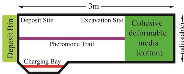
**Fig. 1** Schematic of a table top test bed with adjustable tunnel walls
