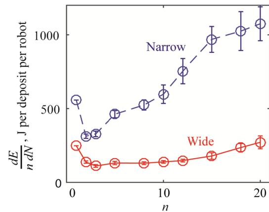
**Fig. 9** The dependence of energy consumption per excavation per robot on the number of robots in the tunnel ( $n$ ) acquired in the simulations in wide (solid line) and narrow tunnels (dashed line). Error bars indicate standard deviations
