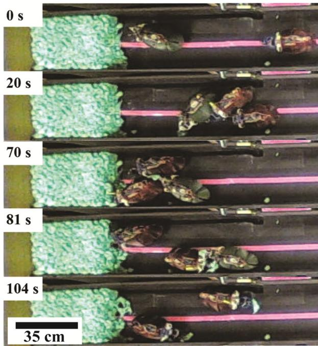
**Fig. 4** Snapshots showing the clogging of three robots in the narrow tunnel (2 BW) near the excavation site
