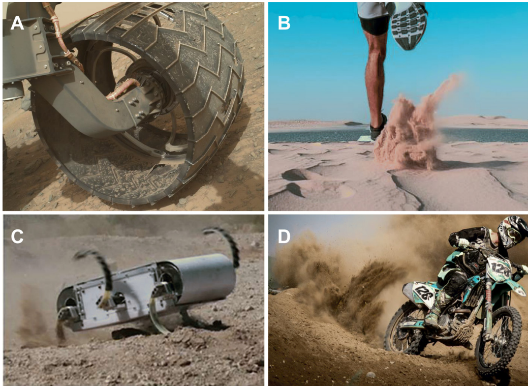
Figure 2.1: Examples of Locomotion on Granular Surfaces at Various Speeds (A) Wheel of the Curiosity Mars rover (Diameter \sim 50 cm) [72] (B) A running human [73], (C) RHex C-legged robot (C-leg limb length \sim 18 cm) [74], and (D) A dirt bike racing through loose terrain (Diameter \sim 50 cm) [75]. [Photo credits: (A) MAHLI Imager on Curiosity , NASA; (B) A. Singh, Pexels; (C) G. C. Haynes, A. M. Johnson, and D. E. Koditschek, University of Pennsylvania; (D) Daniel, Pexels].
