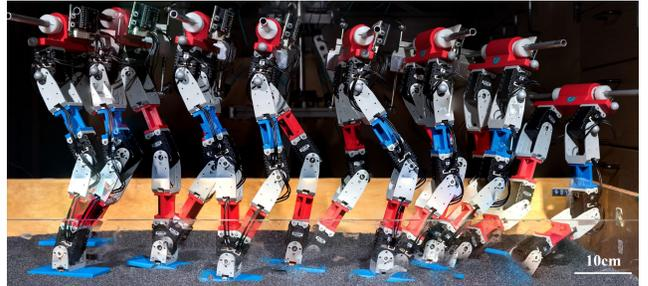
Fig. 1. Time-lapse photograph of a planar biped walking on a bed of poppy seeds, an experimental surrogate for granular terrain. The robot walked at 10 cm/s. Photo credit: Rob Felt [9].
